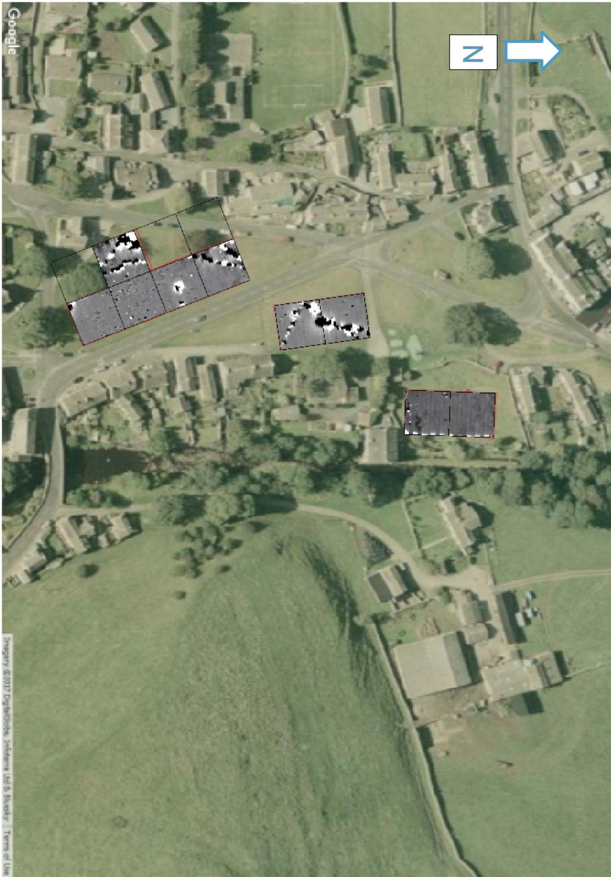
Figure 3 : Bainbridge magnetic survey data superimposed on Google Satellite image
