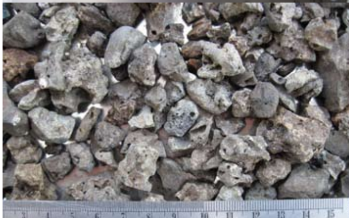
inclusion of dark grey slag with some baked clay and secondary crystallisation on right hand side. Figure 10 (bottom) small slag from F2 after removal of soil by sieving and washing.
