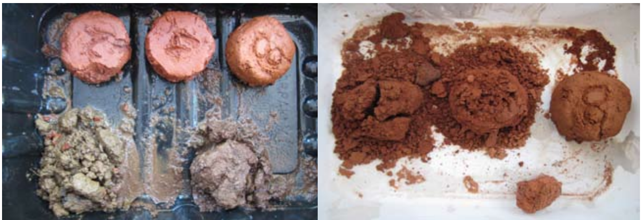
Figure 2 (left). Plugs after soaking in water for one hour. From top left: 500 °C, 650 °C and 950 °C and from bottom left: 105 °C and 210 °C.
