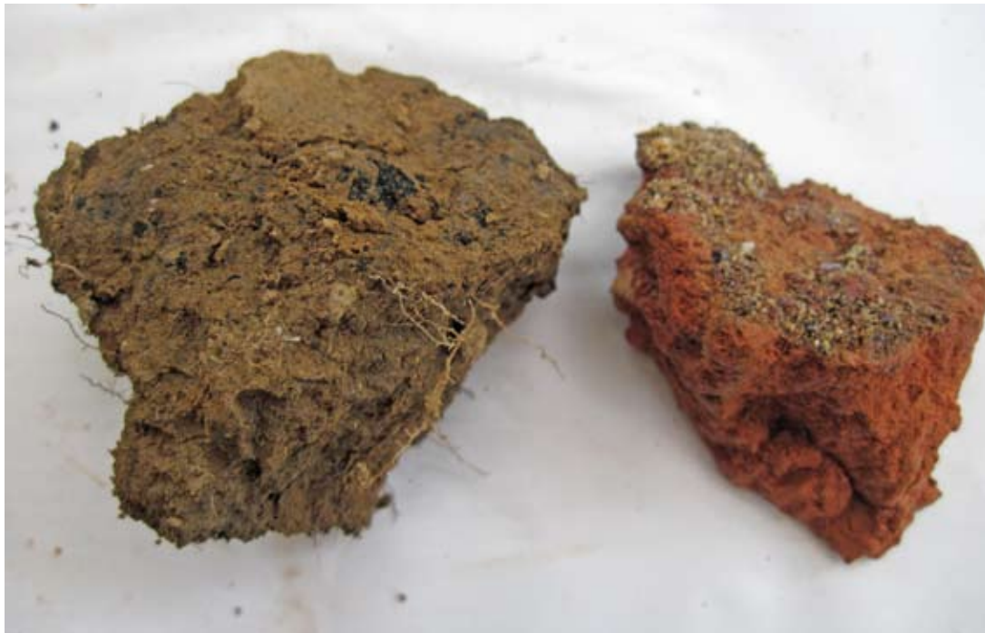
Figure 4. A piece of natural state clay (left) compared with a similar piece which has been heated to 950 °C and slightly moistened.
