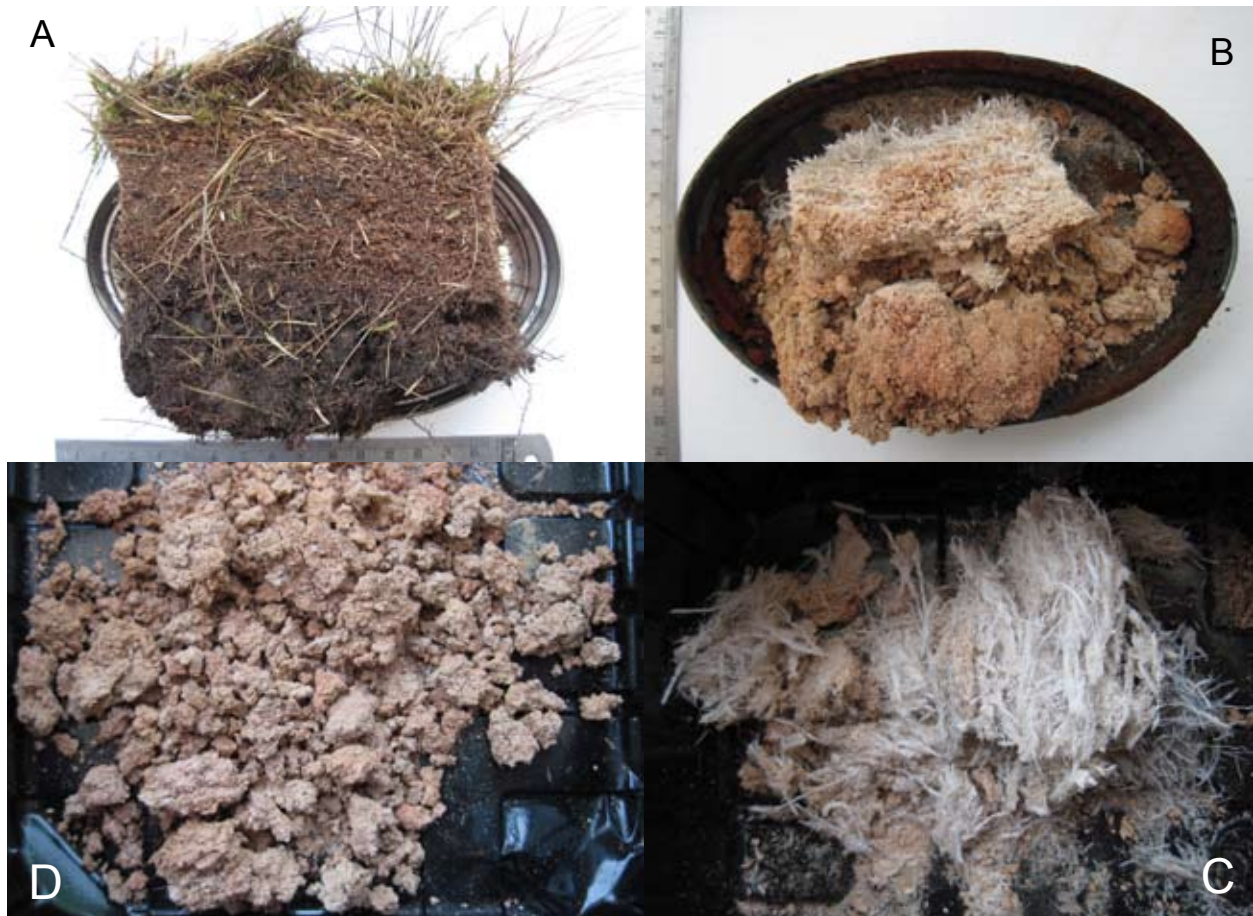
Figure 5. Effect of heat on a piece of turf. (A) Piece of natural state turf. (B) After calcining for 4 hours. (C) Ash formed from the vegetable content of the turf. (D) Residue from the mineral content of the turf.
