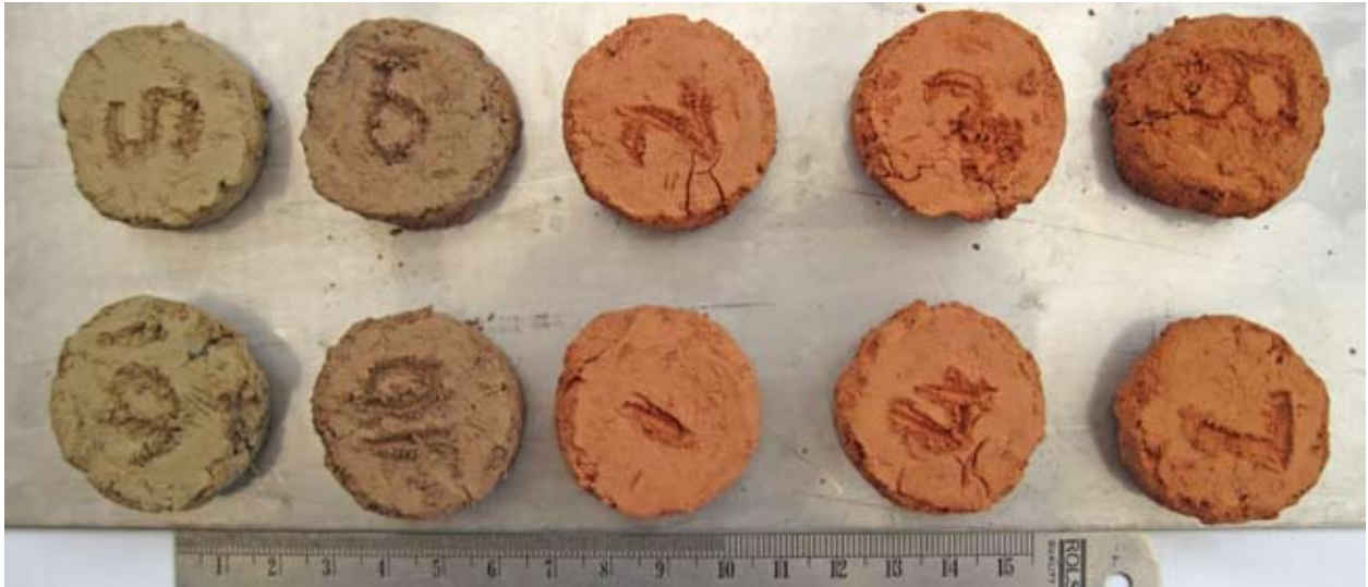
Figure 1. Pairs of clay plugs heated to (from left) 110 °C, 210 °C, 300 °C, 500 °C, 650 °C and 950 °C. The lower row is a duplicate of the upper row. The reddening temperature was defined more closely by a further test and shown to take place between 450 °C and 500 °C.
