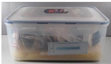
Figure 1. Iron artefacts packed with silica gel in air-tight plastic box with humidity indicator card.
