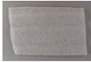
Figure 4. Polyethylene foam; example above is Jiffy foam. Suitable for temporary storage.
