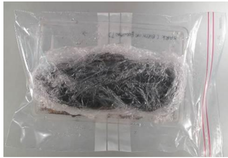
Figure 2. Waterlogged wood wrapped in cling film, double bagged with rigid support.
